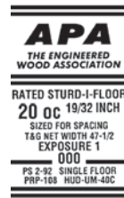
Figure 8.16b Typical grade-trademarks for nonveneer single-layer floor panel. (Courtesy of APA—The Engineered Wood Association.)
