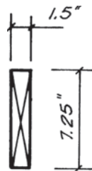
Figure 4.15a A 2 \times 8 is a Dimension lumber size.
